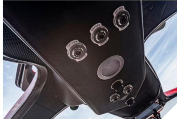
Oxygen system with cannulas and mask
