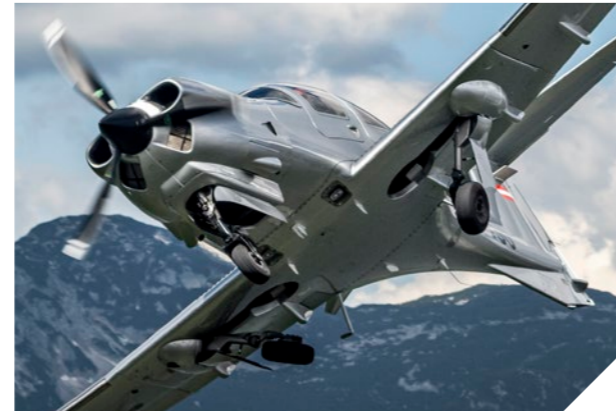
Hydraulic retractable landing gear
