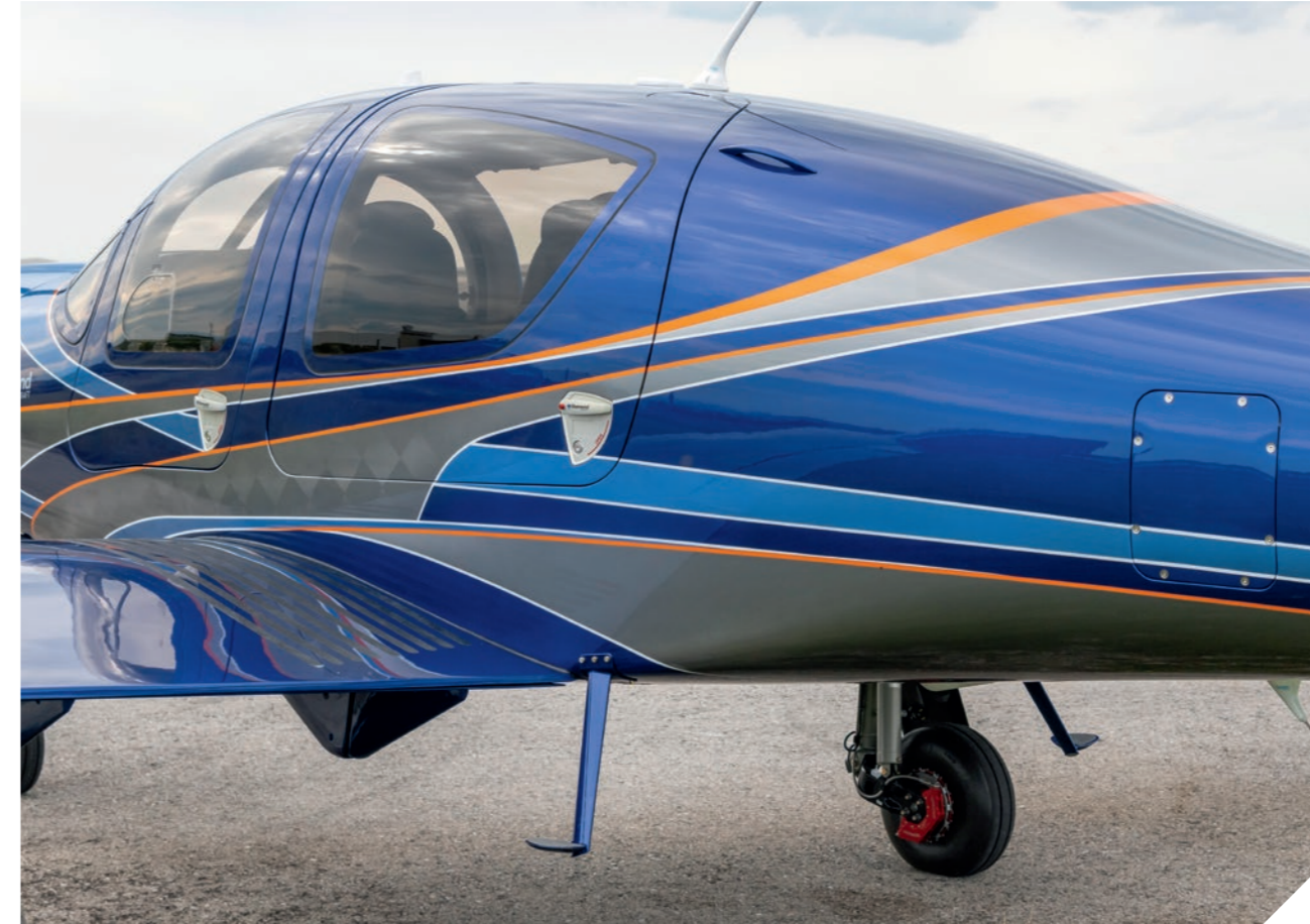
Entry steps and entry grips in aircraft color. Brakes shown in this picture are only of symbolic character.
