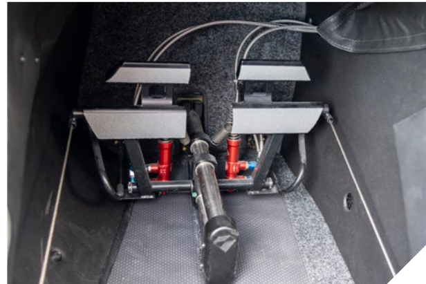
Electrically adjustable rudder pedals for pilot & co-pilot
