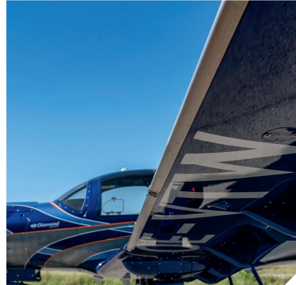
TKS deicing system (TKS panels)
