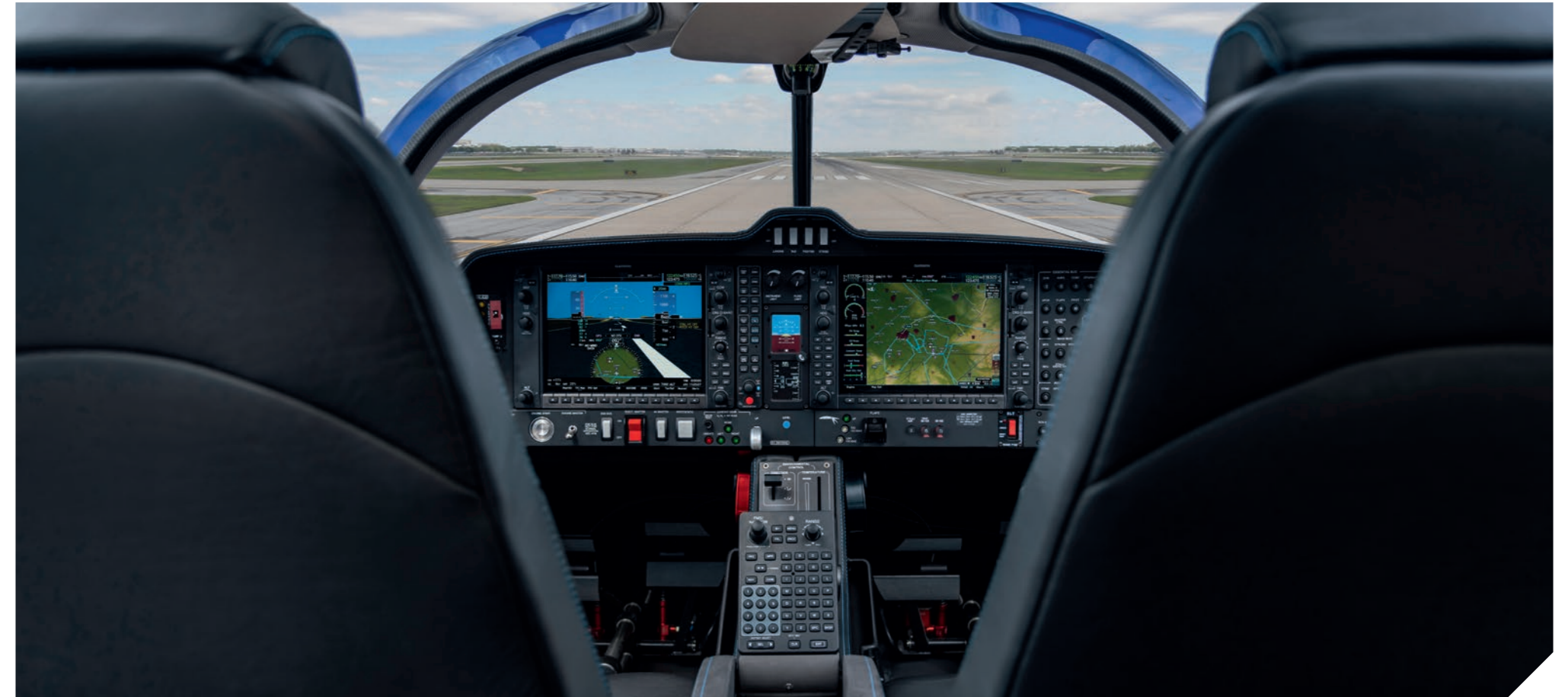
Integrated Garmin G1000 NXi glass panel cockpit
