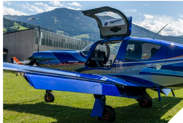
Electrically operated single hinged double slotted flaps
