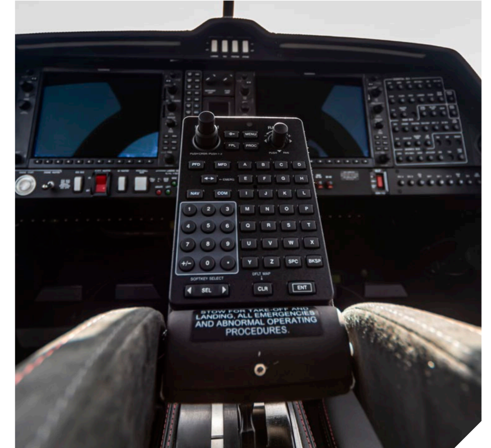
Middle armrest with Garmin GCU 476 keypad
