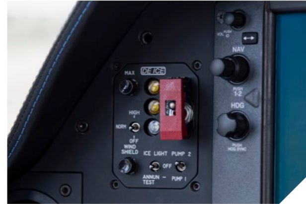
TKS deicing system (cockpit control panel operation)
